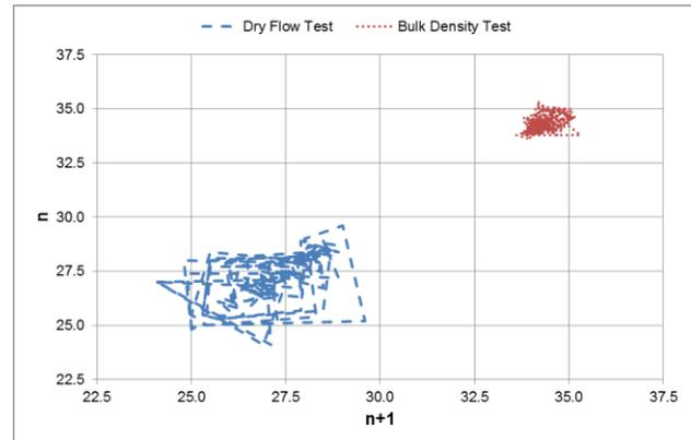
Fig 8: Poincaré Map for Full Data Sets (for LMDPE)
