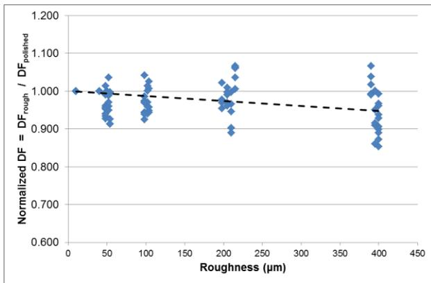
Fig 11: Variation of Normalized Dry Flow with Funnel Surface Roughness (all materials)
