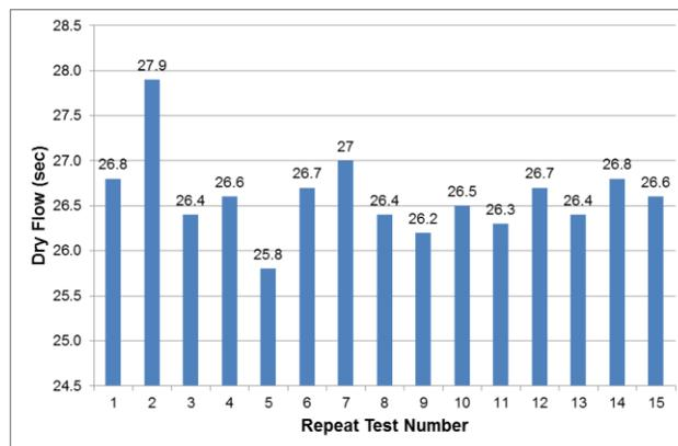
Fig 2: Robustness Test – Dry Flow (LMDPE)
