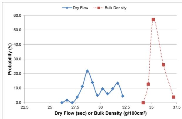
Fig 10: Distribution of Dry Flow and Bulk Density Results (for LMDPE)
