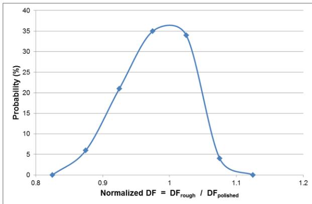
Fig 12: Distribution of Normalized Dry Flow Results (for all materials and all roughness values)
