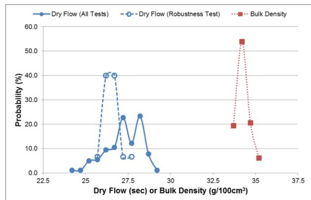
Fig 7: Distribution of Dry Flow and Bulk Density Results (for LMDPE)
