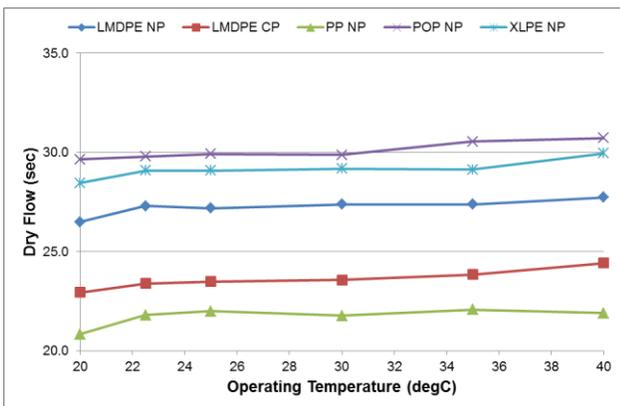
Fig 4: Dry Flow Variation with Temperature
