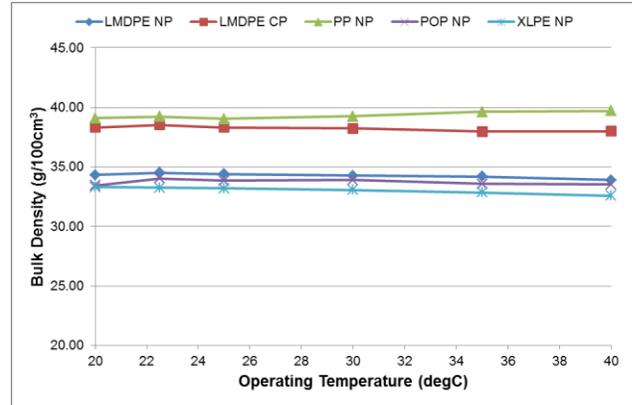
Fig 5: Bulk Density Variation with Temperature
