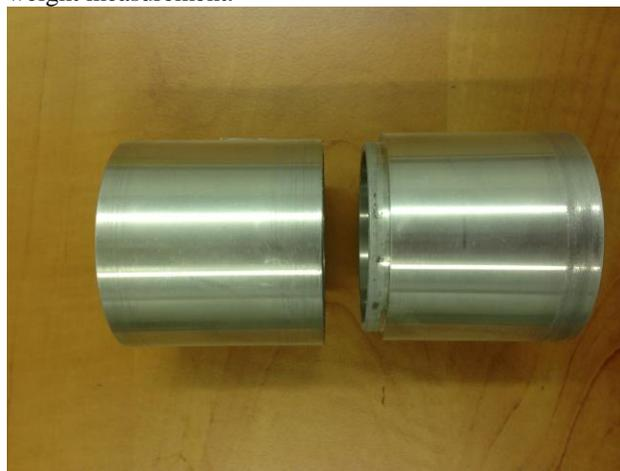
Fig 1: Split Container for Consolidated Bulk Density Determination
